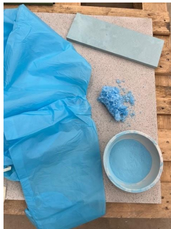
Example of a tile made from recycled glass and used medical gowns
