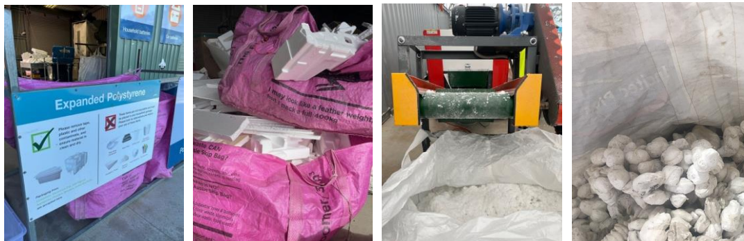
Steps in the EPS processing (L-R): the drop-off point, bags of unprocessed EPS, the granulator, and the product sold into export markets.
