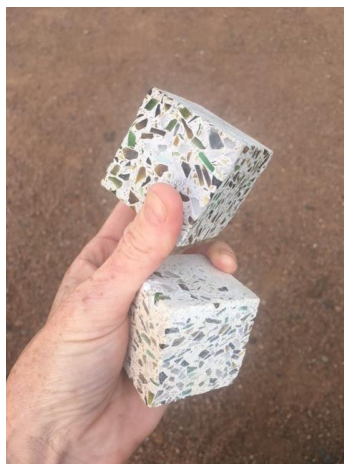
Prototype of a construction product developed in partnership with the University of Western Sydney from 90% glass
